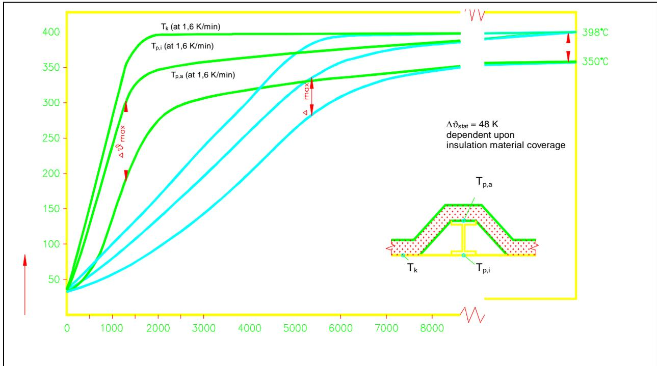
**Figure 3: Temperature increase over time with an IPE 360 profile
