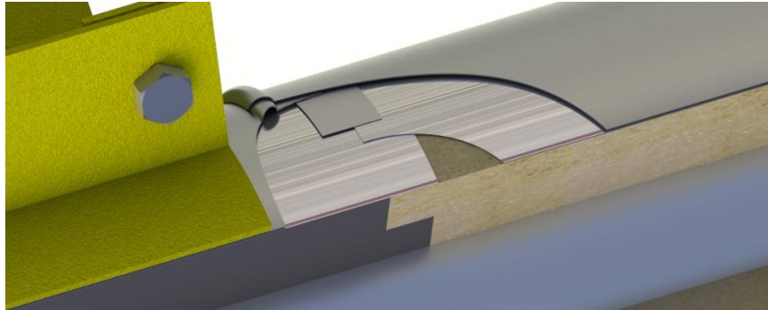
The detail at a pipe support showing how an appropriate pipe support design will allow complete integration of the insulation system of insulation, vapour barrier and cladding to maintain continuity of all three of them.
