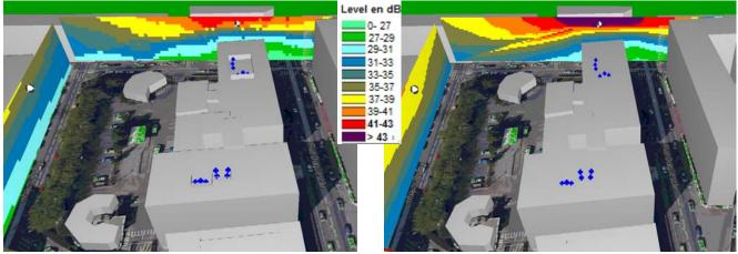
This example shows that screens are efficient in the receiver points, only when they are in a lower or a same level than the sound sources.
